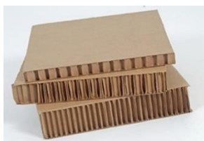
Fig. 1. Composite material based on paper honeycomb
