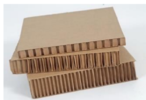
Fig. 1. Composite material based on paper honeycomb
