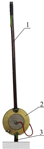
Fig. 7. Prototype of the kinetic energy harvesting system; 1 – seismic beam; 2 – piezoelectric buzzer; 3 – clamping beam
